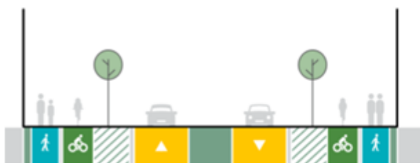
Figure 129: CFAF Outcome - New Connection between Milldale and Grand Drive indicative 24 m cross section
